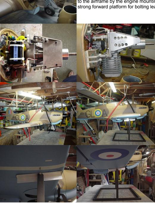
After a rough check on the plane for balance it was obvious I was going to have to add weight to the nose to achieve the desired C of G. I wanted to add as little weight as possible so that meant having the longest nose lever possible. The pictures below show how I have used an old engine mount bolted to a plate and attached to the airframe by the engine mounting bolts to achieve a strong forward platform for bolting lead ingots to.
