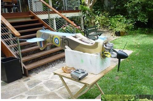
The crankshaft extender and **Vailleyaviation** spinner have been fitted and a **Bolly** carbon 20" x 12" three blader is the prop of choice. The blades are fairly narrow so I am hoping for around 7,000 r.p.m. eventually.
